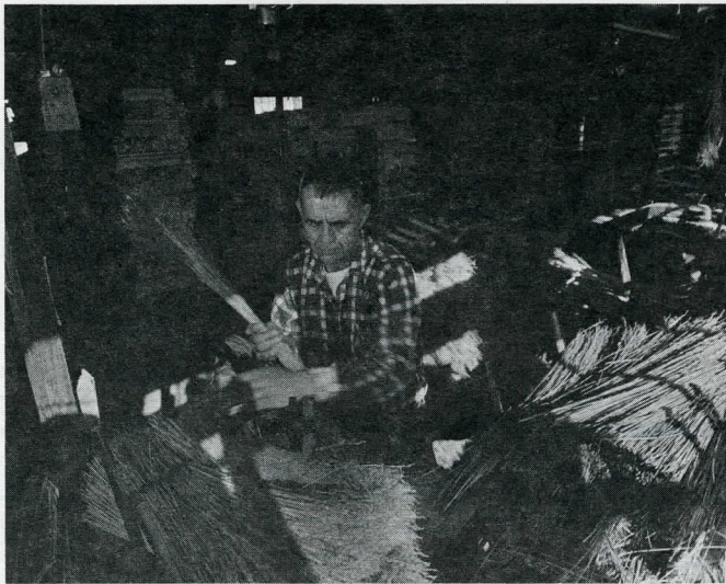
John Ferguson, a broom maker for 30 years, at the floor broom tying machine.
