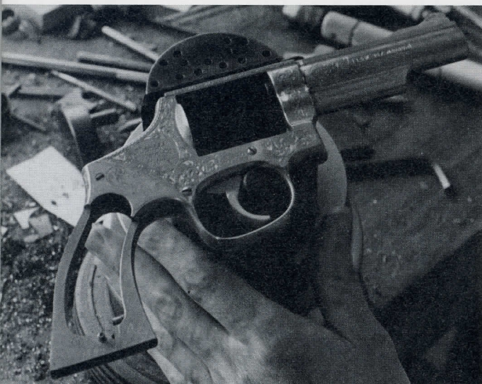
Above: A pistol is stripped of grips and cylinder before engraving begins. Sperry engraved this Smith and Wesson .357 magnum for Wayne County Sheriff Bernie Crabtree. Photo by Michael Holland. Right: The finished product rests in the hands of Sheriff Crabtree.
