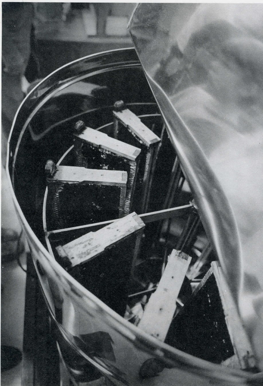
After uncapping, the frames go to an electric separator, where centrifugal force will spin the honey from the comb. Such equipment modernizes the age-old practice of beekeeping.
