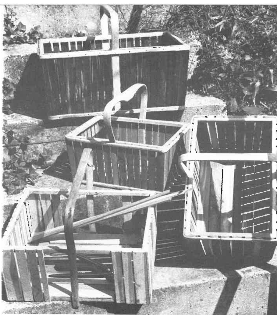
Mr. Richmond's baskets are patterned after those his father made, although of cedar rather than white oak. The slats, frame, and handle are joined by small nails.
