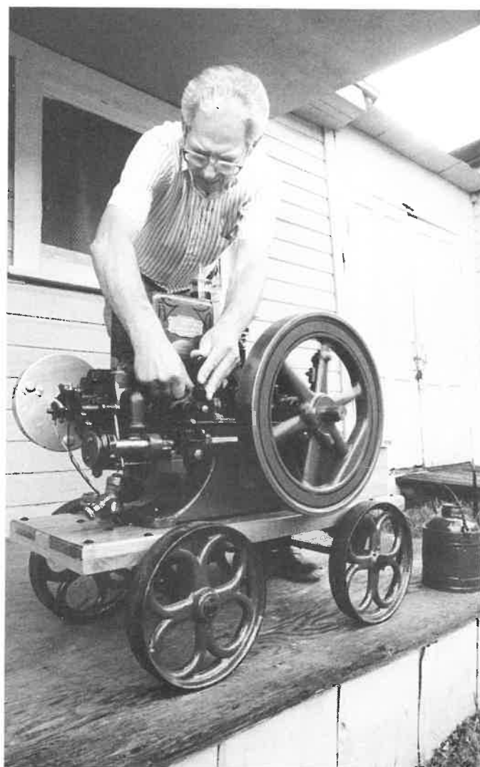
A man and his motor: Restoring the old engines is one job and keeping them running is another. Here Gene Townsend tinkers with his 1.5-horsepower Domestic, as shown in the company's advertisement below. This was Domestic's smallest model, intended for "pumping water, running cream separators, churns or any other light work."
