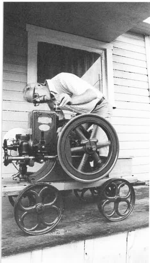
A man and his motor: Restoring the old engines is one job and keeping them running is another. Here Gene Townsend tinkers with his 1.5-horsepower Domestic, as shown in the company's advertisement below. This was Domestic's smallest model, intended for "pumping water, running cream separators, churns or any other light work."
