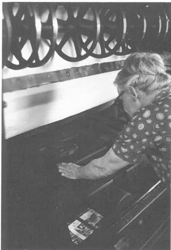
Production of the Times has now been modernized, but employees made daily use of very old printing skills up until a few years ago. In this series of photos from 1983 Eva Grimes hand sets type at far left. Evelyn Withers locks type in for an ad layout, then positions it on the paper's Babcock flatbed press. The final picture shows the fresh imprint, made by the letterpress process with the type actually touching the paper. The Babcock press and Eva are now retired, but Evelyn continues to do letterpress printing for stationery and other job orders.
