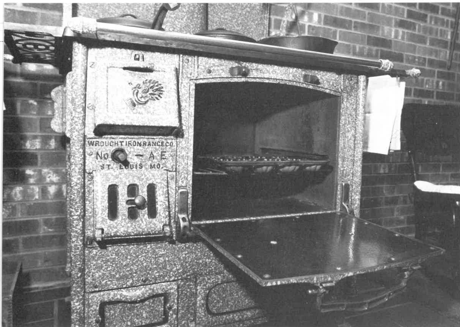
The Home Comfort layout is similar to that of modern electric and gas ranges, with the addition of firebox and ash doors to the left.
