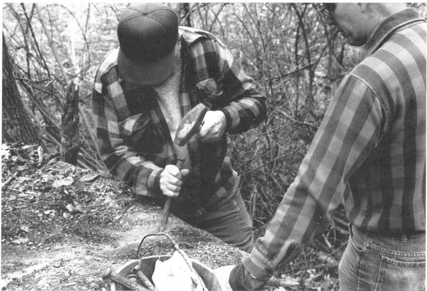
Ben Carr learns stonecutting by the time-tested "watch and try" method. In these photographs, above and at right, Dare Crawford shows how to score a boulder with chisel and hammer, then lets Ben try it.
