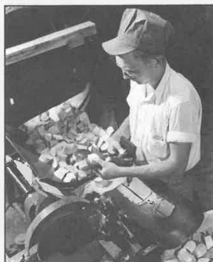
Meadow River manufactured specialty products ranging in size from ships' beams to shoe heels. Precision was important with all of them. John Surbaugh (above) gauges a representative shoe heel.
