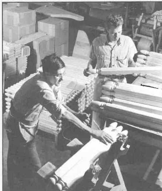
Lumber passed through a variety of other saws and machines after leaving the band saw. These workers (left) check boards leaving a planer.
