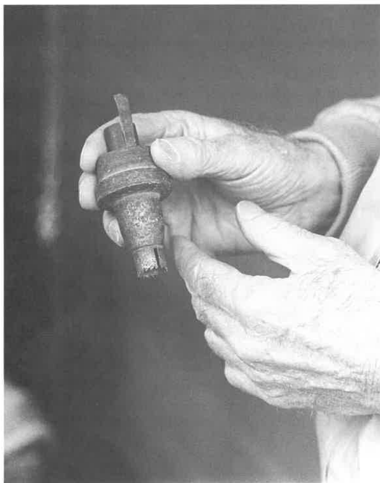
Cutting buttons required specialized tools, including tongs to grasp the shell firmly by the rim. The shell was pressed against the spinning blade of a stationary saw, the idea being to get as many good blanks as possible from each shell. The tubular saw blades, such as the one shown below, were similar to modern hole saws.
