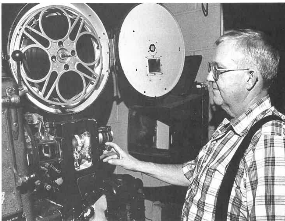
Projection technology hasn't changed much in West Virginia drive-ins. Here projectionist Junior Armstrong (above) shows off one of The Grafton's Super Simplexes, essentially similar to the Super 135's shown in the 1950's picture of the Sunset Drive-In's projection booth. The Sunset projectors are still in daily use.
