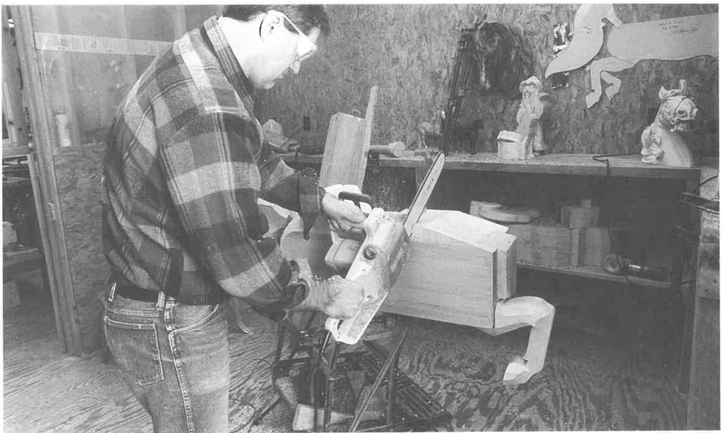
Though detail carving is all done by hand, Garton uses power tools for rough shaping. Early carousel horse carvers used "whatever took the wood away," he says.
