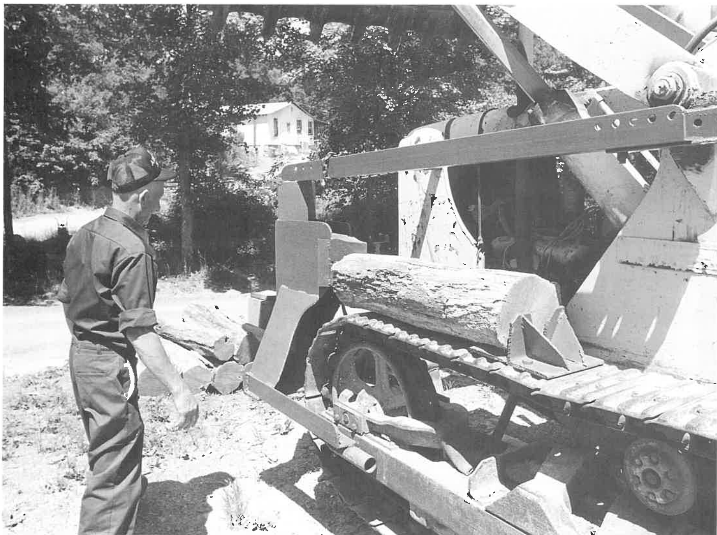
This homemade log splitter has no trouble with man-sized logs. The old end-loader sits on blocks, its tracks rotating freely to carry logs to the big wedge in front.
