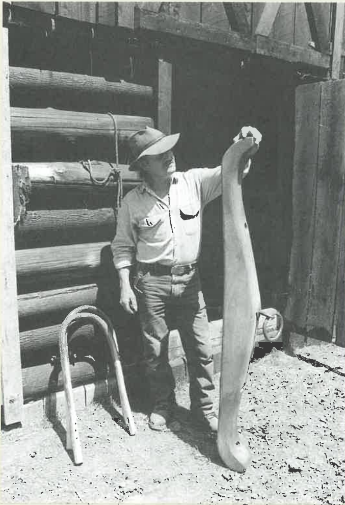
Daniel uses cucumber wood, a variety of magnolia, to carve the yoke for his team. The most challenging part, however, is achieving the 180° bend in the hickory bows. Photo by Michael Keller.
