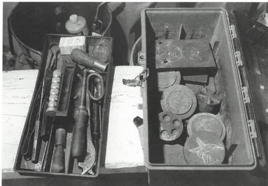
Tools of the trade. Most of what Jennings uses to make his beautiful paperweights will fit in one small carrying case and a bucket. The dies are seen at right, and the hand tools are in the tray at left.
