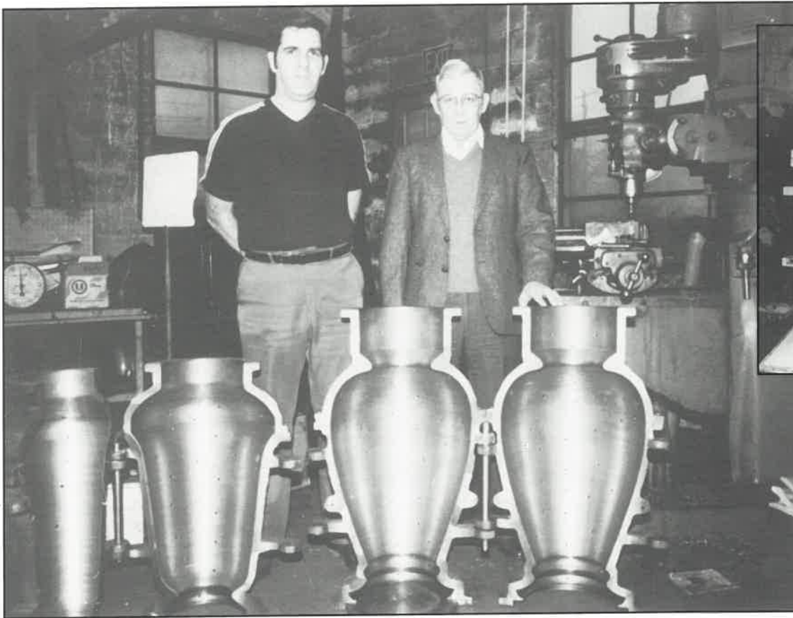
Employee Matt Linger at left stands with Paul in Weinberger's Mould Shop in Weston, during the 1980's. The large, two-piece metal moulds shown here are made from intricate, handmade wooden patterns (inset). Photographers unknown.
