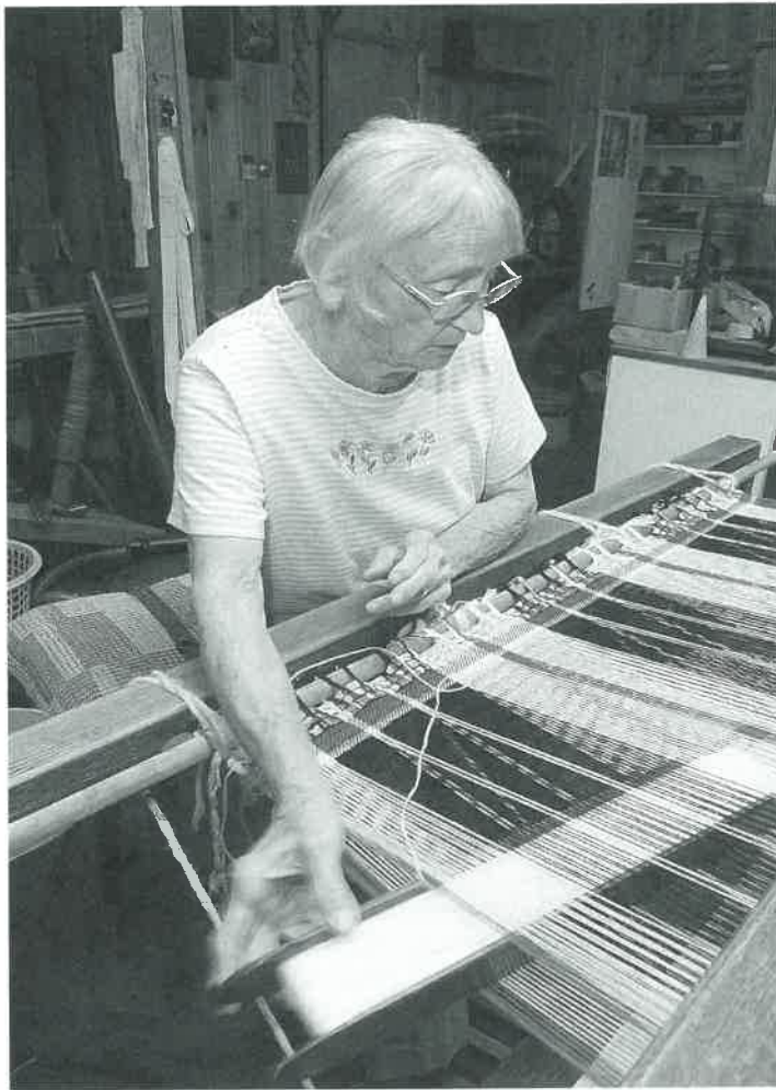
Dorothy passes the shuttle through the shed — an opening formed between the long warp threads, which are strung lengthwise on this loom. The crosswise threads are called the weft. Photograph by Michael Keller.
