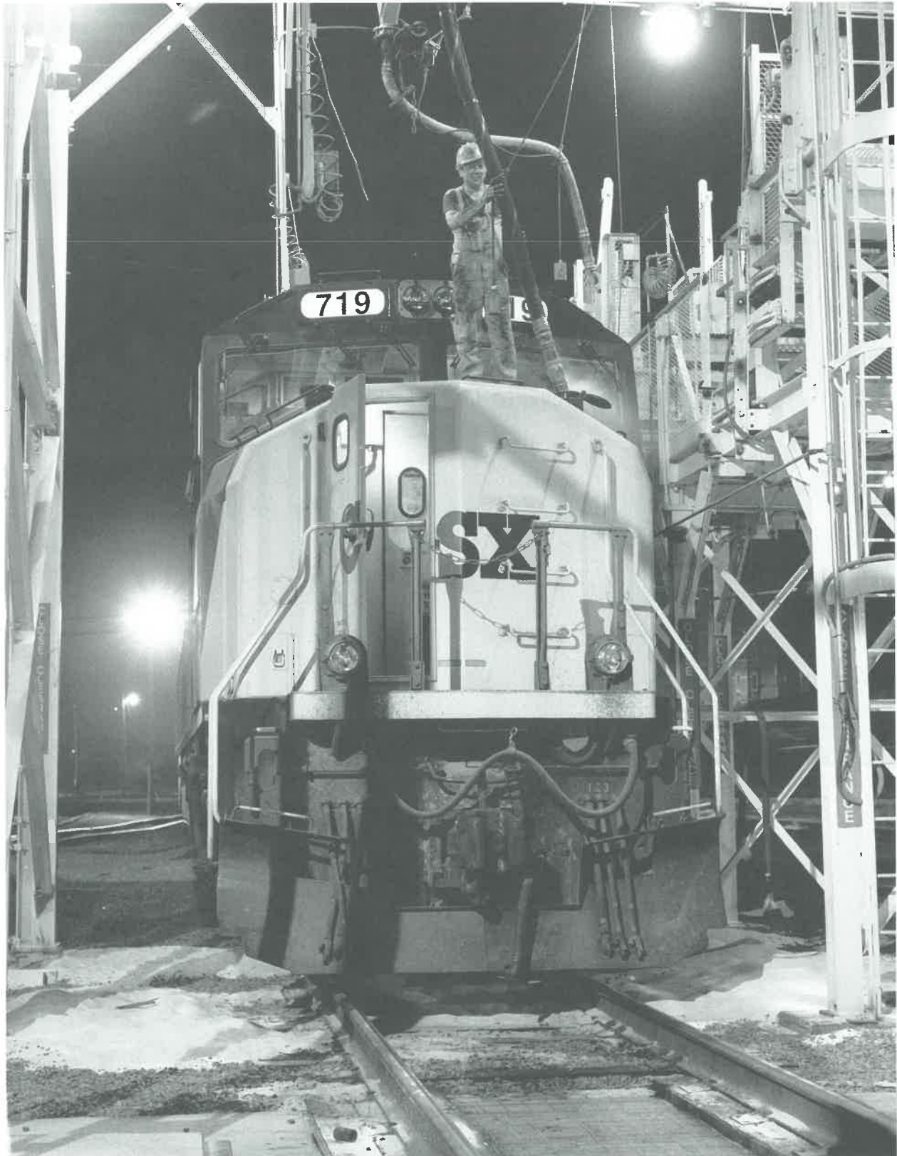
Machinist Joe McKinney loads sand into a locomotive as part of routine servicing in the Grafton yard on August 8, 1998. The sand will be applied beneath the locomotive's wheels, helping the engine gain traction on steep grades or in adverse weather conditions.
