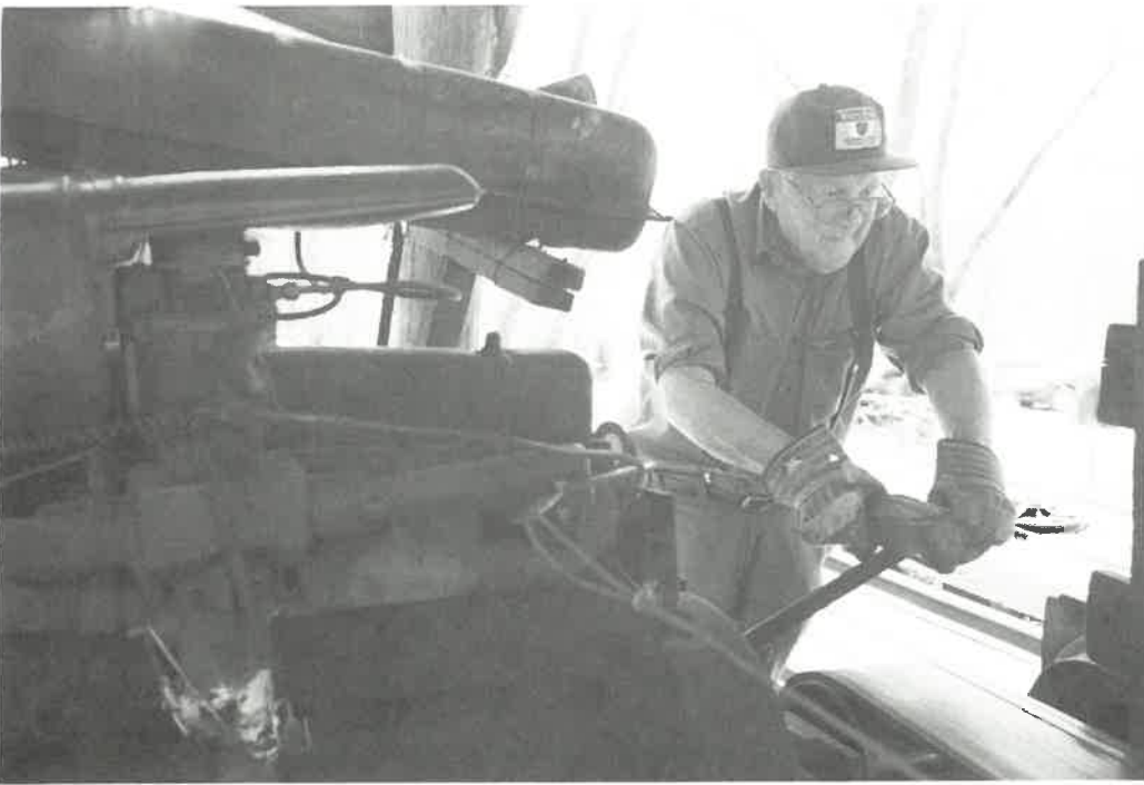
John Hahn, 82, dresses a belt on the brothers' sawmill. The motor is from a 1949 Buick Roadmaster.
