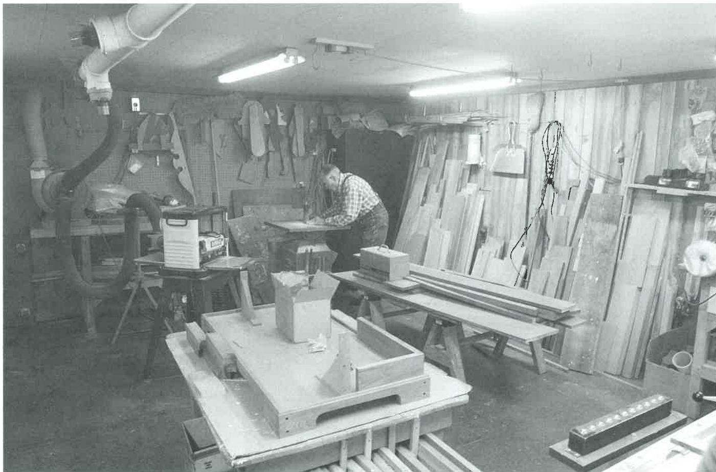
Rube at work in his shop. The hoses are part of his dust exhaust system.
