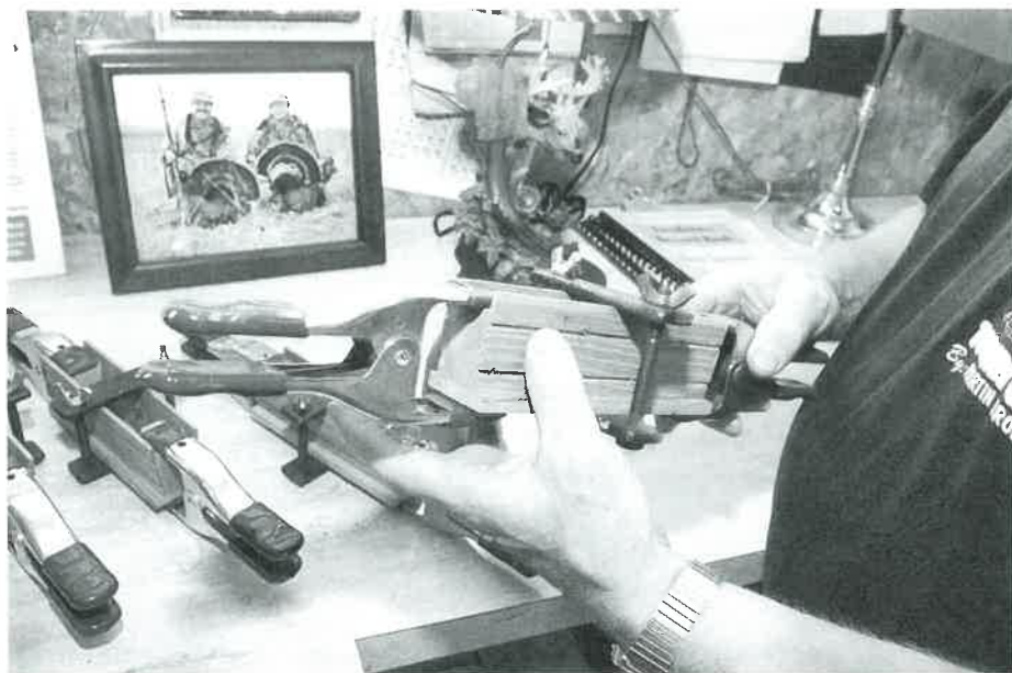
Clamps hold bottom boards to the core blocks of several new box calls, as Peck sets them aside for the glue to dry. Once finished, these calls will sell for prices ranging from $26.95 to $200. For more information, call (304) 233-5518. Photograph by Michael Keller.
