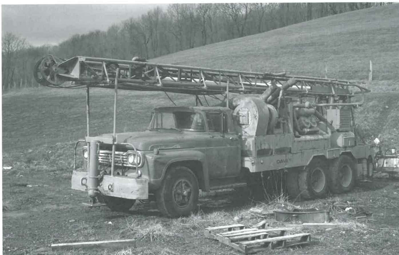
Keith Wotring's drilling rig. Keith has drilled more than 100 wells and says he can go down as far as 300 feet with this equipment.
