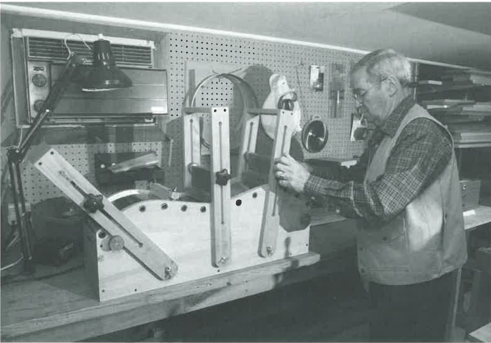
Resourceful and imaginative, Bernard sometimes wakes up at night with an idea for a new tool or device for his woodshop. Bernard designed and built this innovative tool, used to bend the sides of a dulcimer.
