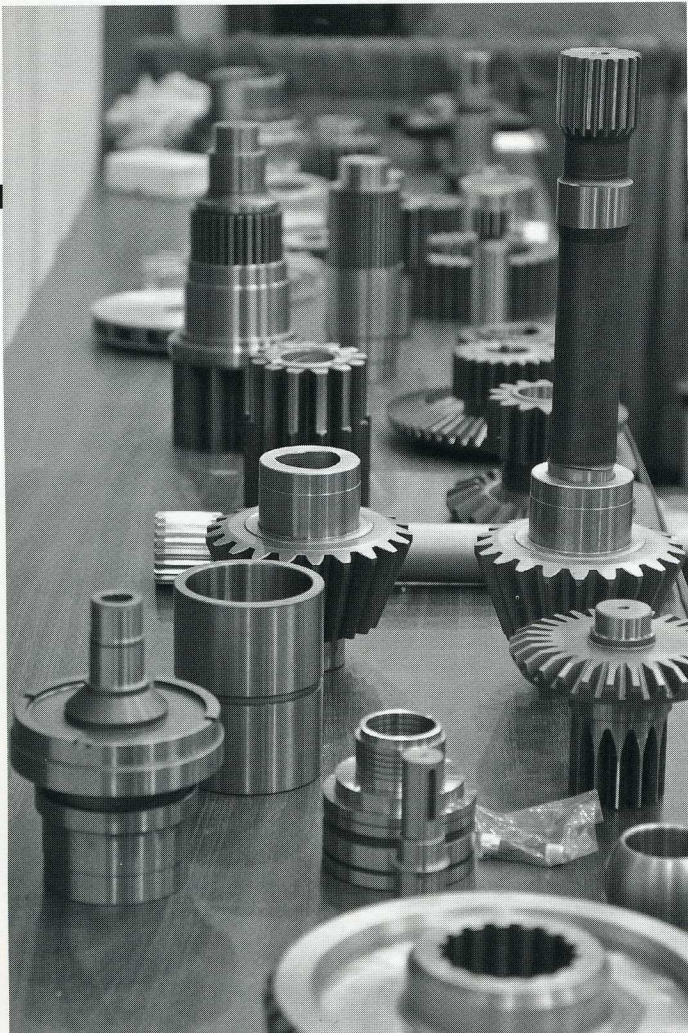
These gears, shafts, and sprockets are custom-made to replace worn parts in a variety of mining machines. After-market replacement parts were in abundance at the Bluefield Coal Show.
