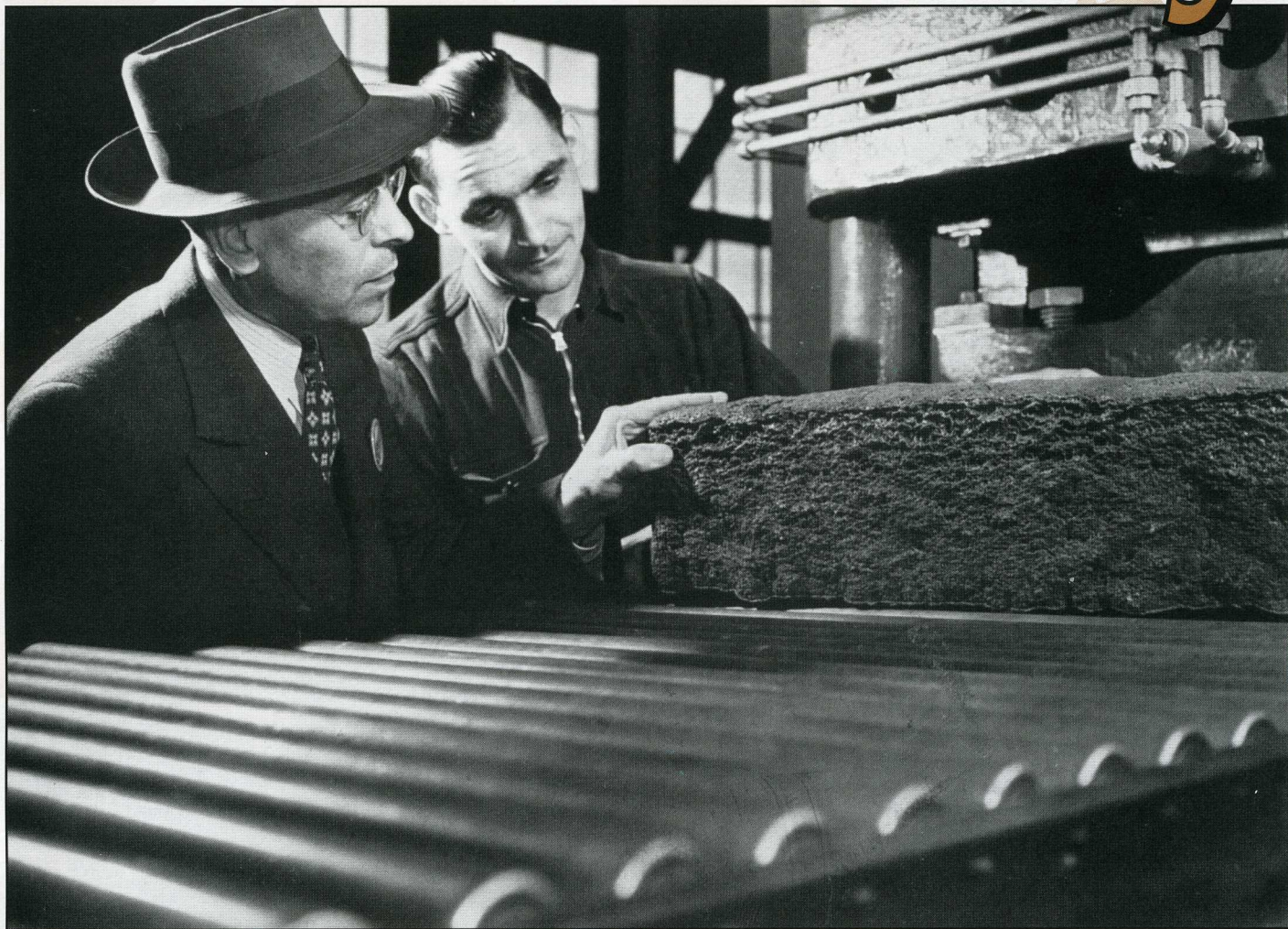
A 75-pound bale of synthetic rubber — the finished product — emerges from the hydraulic press. The Institute Plant produced 90,000 tons of synthetic rubber annually. Here plant manager George Graham, at left, and an unidentified worker inspect a finished bale.
