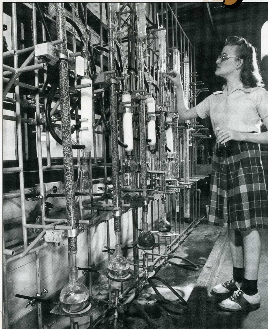
A laboratory technician checks the distillation units in the control laboratory at the Carbide plant. Butadiene was made from grain alcohol, and styrene was made from benzene and ethylene gas. They were then combined to make Buna-S rubber.
