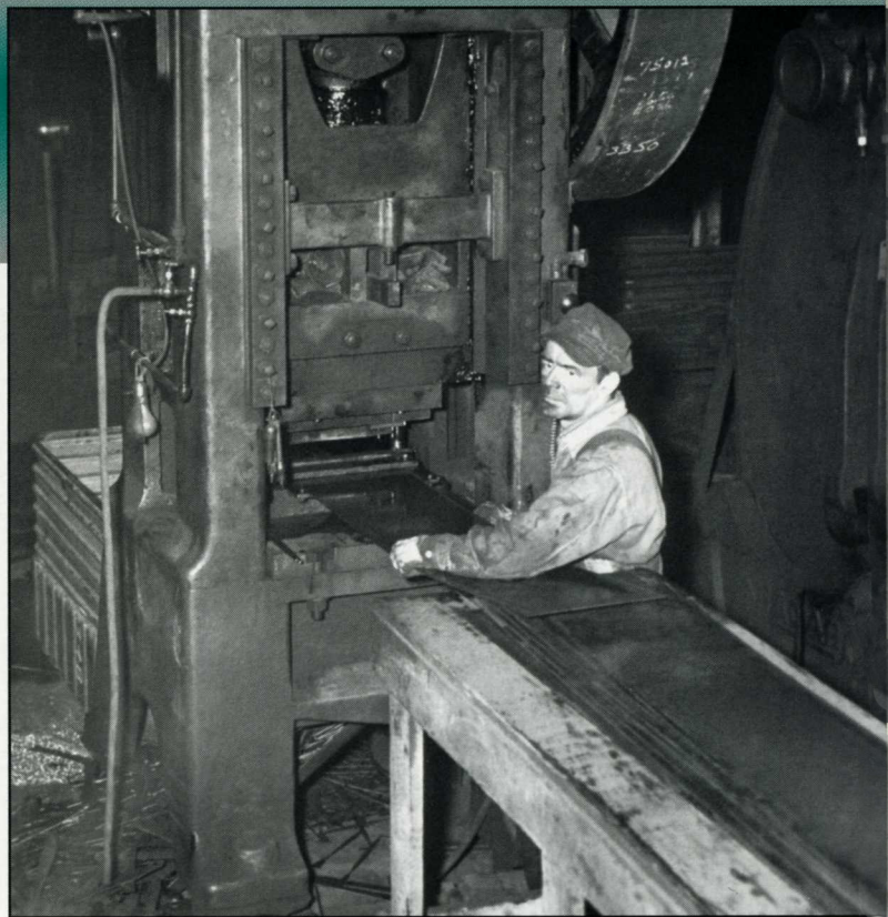
A Kelly employee operates a large shear at the axe plant in Charleston. It is likely the steel being cut here was used to make shovels. Photograph courtesy of West Virginia State Archives, Ross Noble Collection.
