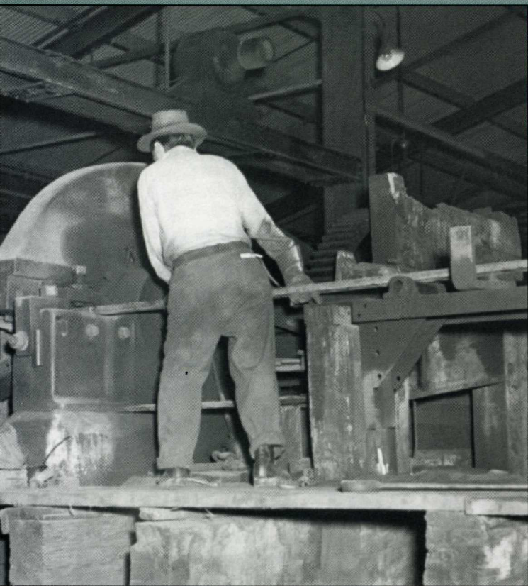
A man feeds a length of metal bar into a cutting machine, possibly producing blanks for axe or other tool heads. Photograph courtesy of West Virginia State Archives, Ross Noble Collection.
