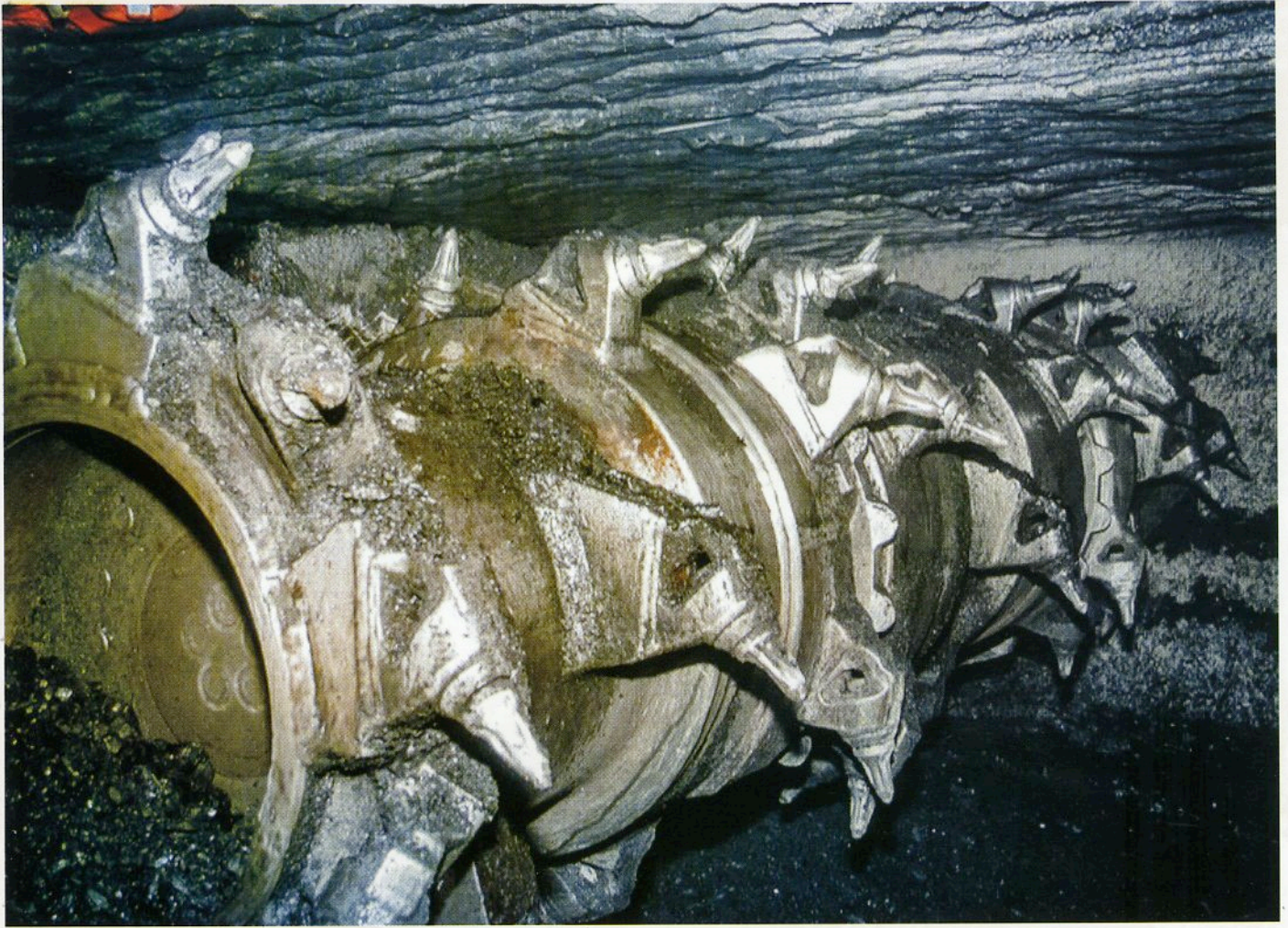
Revolving "ripper" head of a continuous mining machine. All photos courtesy of the author.
