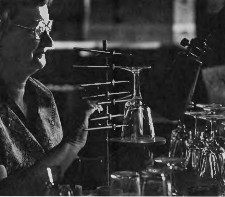
Nora Weaver prepares goblets for cutting. Crystal cutters work from only a few guide lines, which indicate the general boundaries of a pattern. Photo by Ron Rittenhouse.
